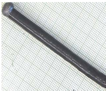
Fig. 5. Bi 2 Sr 2 CaCu 2 O 8+d 0.2 mm/h growth Fig 6 La 1.925 Ba 0.075 CuO 4 0.1 mm/h growth.
