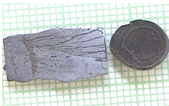
Fig. 3. Cross-section of beginning of crystallization of \text{Sr}_{1-x}\text{Ca}_x\text{Cu}_2\text{O}_7 (grain growth and core visible) [7].
