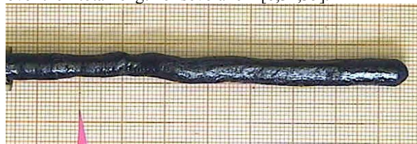
Fig. 7. SrCu 2 (BO 3 ) 2 crystal grown 0.22 mm/h in 2 atm of O 2 . Beginning of the growth marked.
